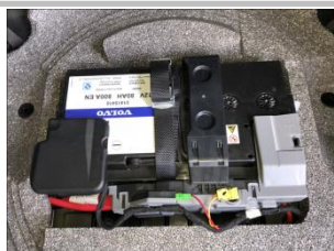
3.5 接正极线：用我司撑杆正极接原车电瓶正极螺栓
