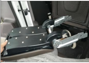
1.7 握住手扶箱钣金,将整个手扶箱取下;
